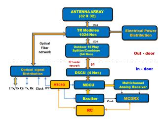
Figure 1. Functional block diagram of the active array MST radar.
