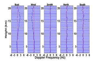
Figure 5. Height profiles of Doppler spectrum observed in the five beams in DBS mode
