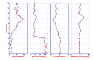
Figure 6. Comparison of winds obtained by AAMSTR with co-located GPS Radio Sonde on 23<sup>rd</sup> August 2017.
