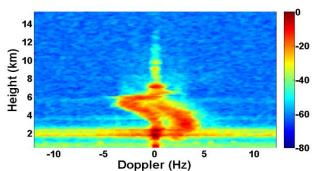
The capability of the radar to observe precipitation events has been explored. Rain event on July  $19^{\text{th}} 2017$ captured by AAMSTR has been shown in figure-10. In order to observe the data from the lower height, the flexible configuration of the antenna array to select one fourth of the total system where 256 elements in 16 x 16 configuration with 2us pulse width has been used.
